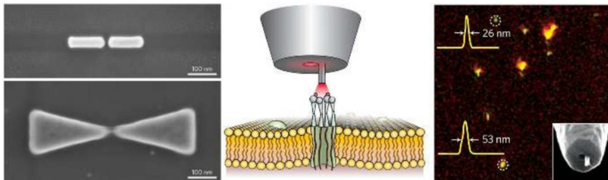
Left panel: two antennas with gap sizes down to  $\sim 10$  nm, fabricated by focused ion beam milling. Center panel: schematic illustration of a biological imaging with optical antennas. Right panel: Fluorescently labelled antibodies imaged by the antenna probe.<sup>1</sup>
