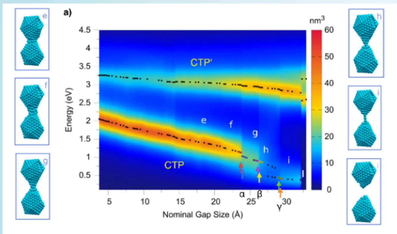
Optical response of metallic nanojunctions driven by single atom motion
